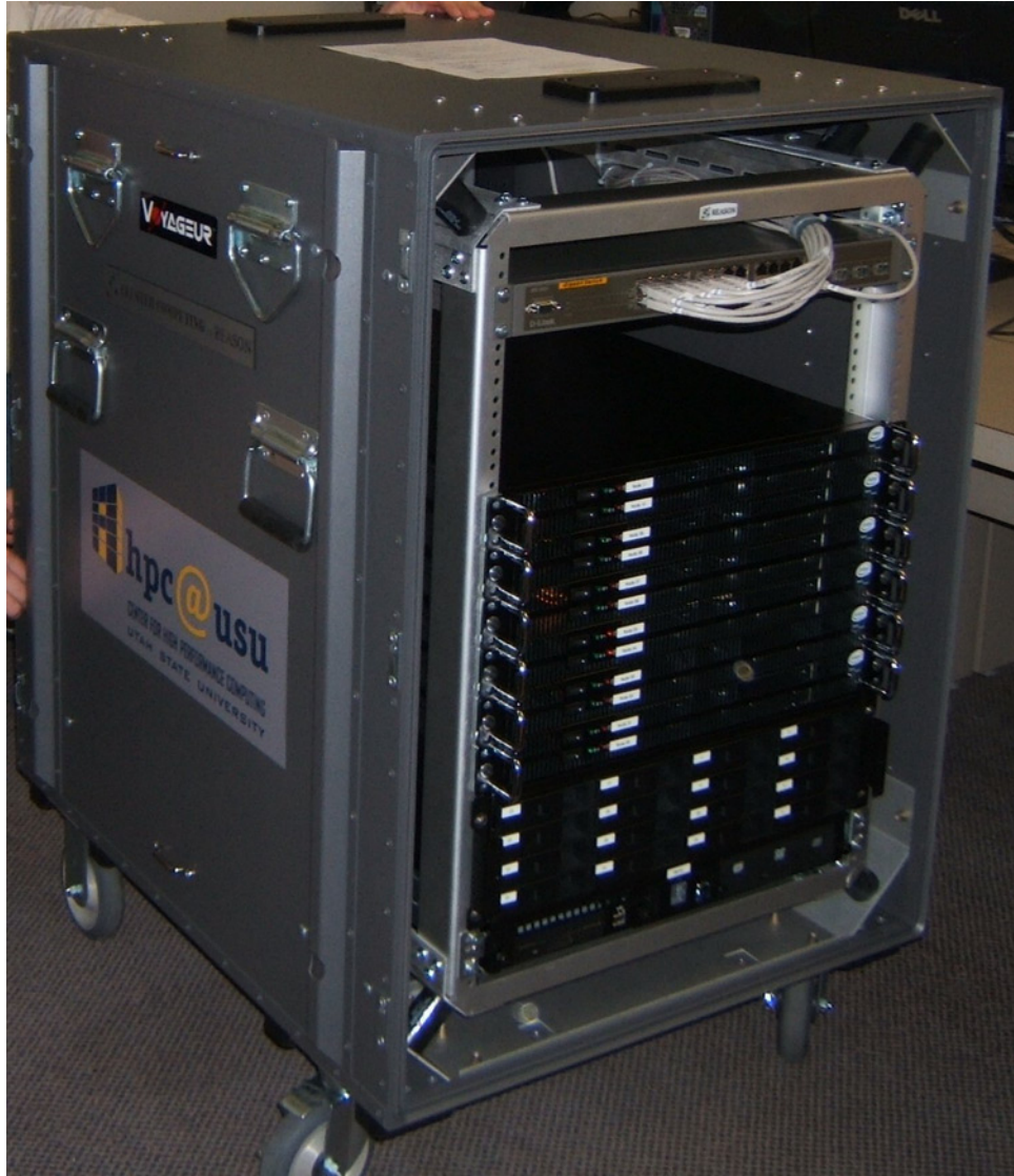
Fig. 3 The implementation of the low-power PIV cluster supercomputer.
